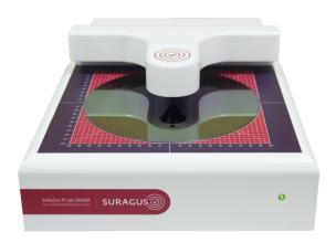
By modulating the emission frequencies of the initial magnetic field, we will be able to control its depth of penetration and therefore the thickness of the layer that we wish to measure. It is therefore possible to perform measurements of one or more layers simultaneously on a wide range of materials such as metals, glasses, thin coating layers, conductive films, electrode layers, papers and textiles. conductors, or even polymers.
